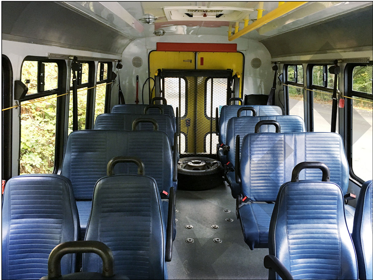
Figure 3.6 – Pender Island community bus interior with rear-mounted wheelchair lift
